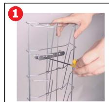
Loosen 1 screw holding the top back plate in place. Remove the other screw from the unit and let back plate hang down. Take same steps for the bottom back plate.
